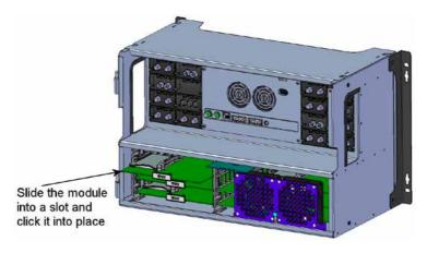
**Note** You can use hot swapping when you insert a module into or remove a module from the TDX system.
