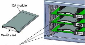
CA modules and smart cards inserted in the output modules
