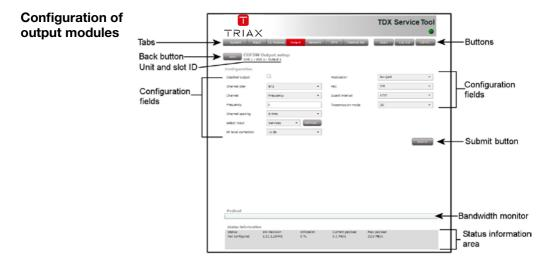
The first time the TDX Service Tool displays the Configuration window for an output module in a new configuration the fields in the window will either display a default value or be empty.
