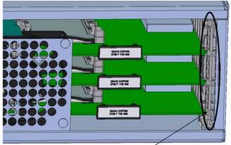
To take a module out of a slot in the output section, tip the lock mechanism and then pull the module out
