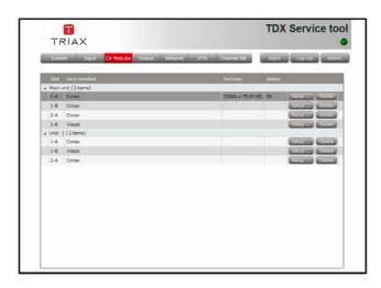
Remember to click the Apply button in the upper right-hand corner to save new settings in the configuration.
