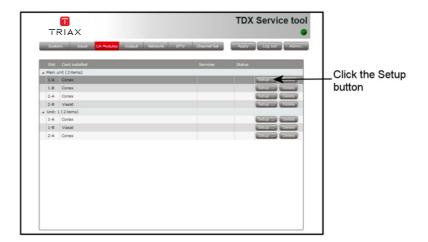
CA Modules con- The first time the TDX Service Tool displays the Configuration window for a figuration window CA module in a new configuration the fields and radio buttons display default values and nothing is selected in the service list area.
