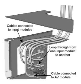
When you connect the cable to the input connector on the AV module, remember to tighten the screws connecting the AV plug to the connector.
