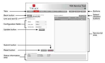
The first time the TDX Service Tool displays the Configuration window for an input module in a new configuration, the fields will display default values and the list of services will be empty.
