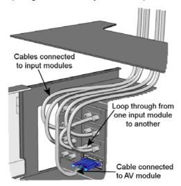
When you connect the cable to the input connector on the module, remember to tighten the screws connecting the AV plug to the connector.
