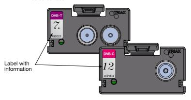
On the bottom of the module you will find a label with the bar code and a serial number printed on it.
