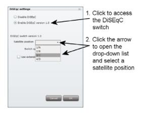
In case your DiSEqC switch does not support vertical (13 volts) / horizontal (18 volts) polarisation and High Band / Low Band frequencies, click the Use extended position/polarity check box to enable up to 16 positions.
