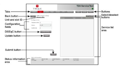
The first time the TDX Service Tool displays the Configuration window for an input module in a new configuration, the configuration fields and the list of services will be empty or display default values.
