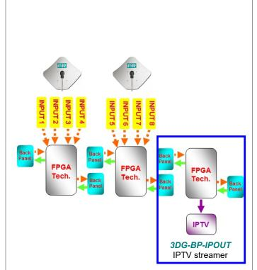
The new **3DG-BP-IPOUT** encoder is able to manage a very high speed IPTV multicast traffic (up to 1 Gbit/s) coming from the Back-Panel and streams all the selected UHD, HD, SD or Digital Radio programs through the Ethernet network (*NOTE: the Ethernet network must obbligatory support the IGMPv2 or higher traffic*)
