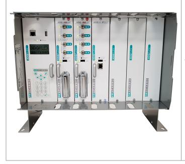
Example: 3DGFlex Evo headend composed by 2pcs of 3DG-4S2-BP quad DVB-S2 receivers and 1pc of 3DGBP-IPOUT IPTV streamer
