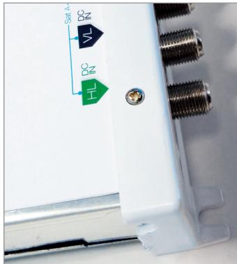
GB: The amplifier can be feeded by trunk lines, the voltage has to be within 13V and 14V; if it is used an higher voltage (ex. 18V) the amplifier will be damaged.
