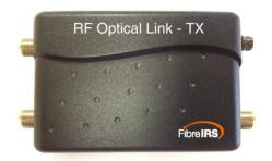
The RF optical link system has been designed to allow one satellite polarity with FM,DAB and DTT to be distributed over s ingle fibre. For additional polarities extra transmitter units can be daisy chained together (Maximum 4) from one power supply. This enables one satellite to be distributed over 4 fibres.
