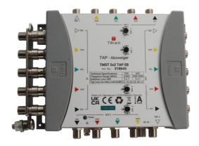
The TMST 5x2 TAP EB is a 5-input two-way tap designed to be used in cascade systems to split the received signals to several trunk lines.
