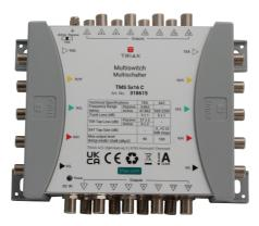
Cascade multiswitch for 1 Satellite position with 5 inputs and 5 trunk outputs, suitable for distributing satellite and terrestrial signals in small to large sized systems. Available with 16 subscriber outputs and powered by the TMS PSU external power supply either directly or via the SAT trunk lines.
