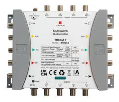
Cascade multiswitch for 1 Satellite position with 5 inputs and 5 trunk outputs, suitable for distributing satellite and terrestrial signals in small to large sized systems. Available with 8 subscriber outputs and powered by the TMS PSU external power supply either directly or via the SAT trunk lines.
