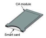
You can insert 8 Conditional Access Modules (CAM) into the TDcH
