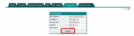
The settings of the IP address, subnet mask, gateway and DNS (Domain Name System) must be adapted to the local network. The IP parameters are updated and activated immediately after clicking the "*Update*" button.
