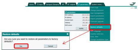
A confirmation message will be displayed on the screen to confirm loading of factory settings. After pressing the button "**Yes**", all settings will be reset to the default values and all streams and logs will be deleted. The factory settings can also be loaded by pressing the reset button (6) for 4 seconds. This feature is available as of software version 1.03.
