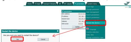
A confirmation message appears on the screen to confirm the restart. After pressing the button "**Yes**", the restart will be done. As soon as the device is ready for operation, the login window appears on the screen. The device can also be restarted by briefly pressing the reset button (6).
