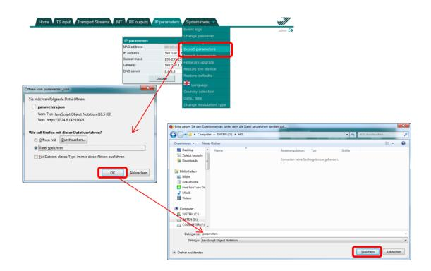
After pressing the button "**OK**", the folder structure will be opened and the storage location for the parameter file, can be selected. To finish saving, press the button "**Save**" (Speichern).
