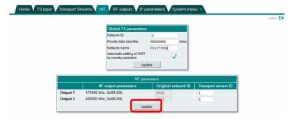
The item "*Network ID*" is a network identification that depends on country, operator and network type. Exact values can be found at <a href="https://www.dvbservices.com/identifiers/network\_id">https://www.dvbservices.com/identifiers/network\_id</a>.
