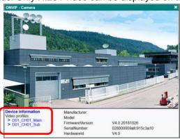
On the left side is the menu of ONVIF. Under "**Device information**", all information about the camera will be displayed. Below this line, all the video profiles that the camera has are listed. By clicking the title of the profile, all parameters of the stream will be listed on the screen.
