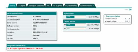
In the device description "**Device information**", the most important information about the device will be displayed. The table displays the device type, current selected modulation type, serial number, installed software version, hardware version, time, country and operating hours.
